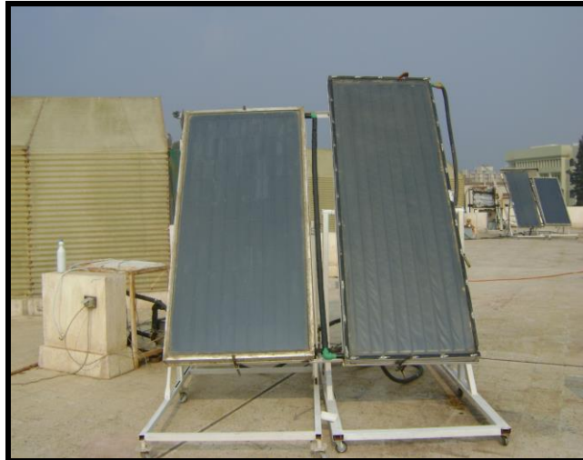
Fig. (1): Solar collectors array, the first one is 2.0 m high and 1.0 m wide giving a net surface area of 2.0 m^2 , the second is 2.4 m high and 0.85 m wide giving a net surface area of 2.04 m^2 .
