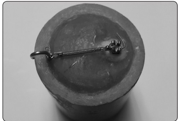
Fig. (1) Orthodontic bracket subjected to 150 gram of force via coil spring.
