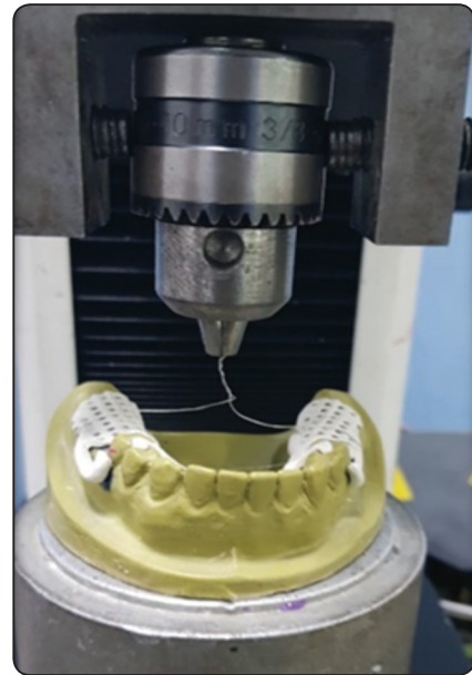
Fig. (5) Framework in universal testing machine
