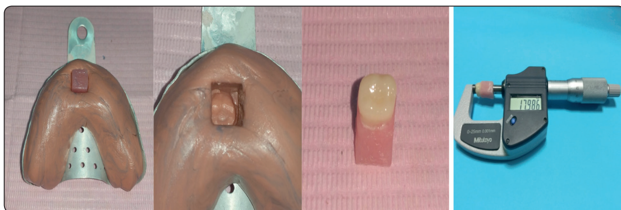
Fig. (1) Duplication of acrylic cylinder with bonded Ker 1 st molar artificial tooth & Digital micrometer measuring the height of the cylinder with bonded tooth
