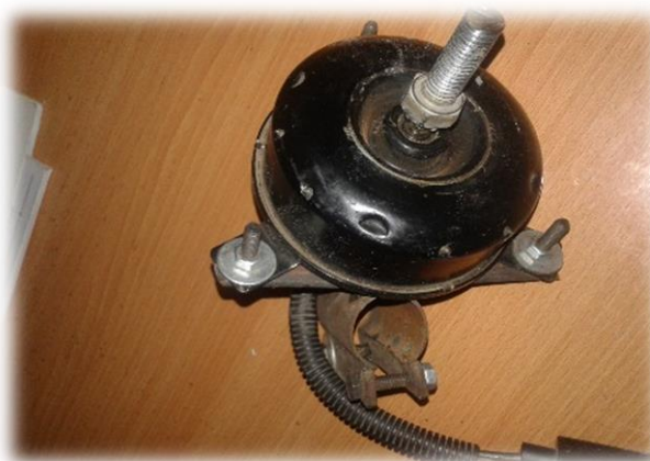
Fig. 4. DC motor installed directly with cutter disk by modified drive shaft
