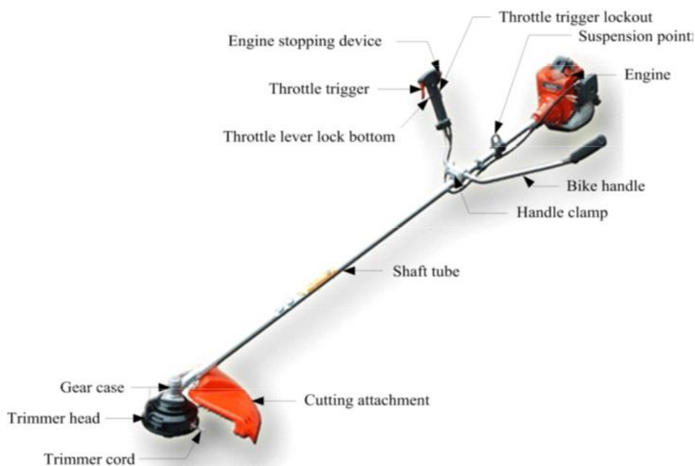
Fig. 1. The main parts of the gasoline-powered disk mower
