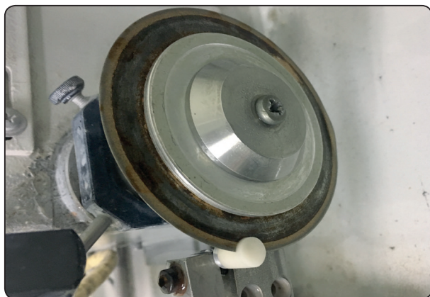
Fig. (1) Cutting ceramic block into disc shaped samples using electric isoMet 4000 micro-saw.
