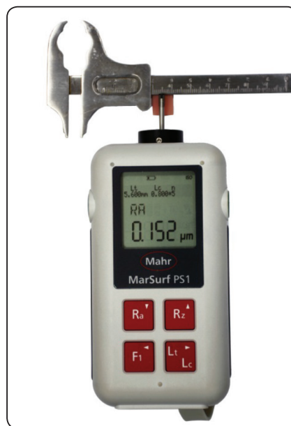
Fig. (1) Surface roughness measurement using pocket profilometer device
