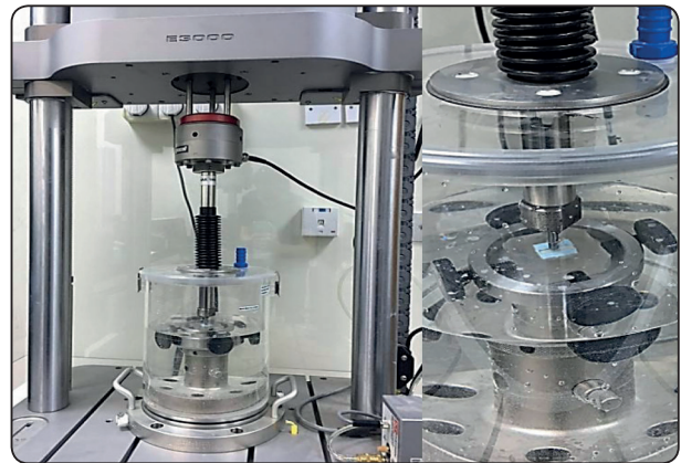
Fig. (1) Universal testing machine used for mechanical cyclic loading
