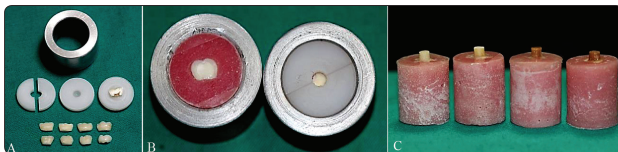
Fig. (2) Cylindrical aluminum mould, a disc longitudinally split at the central hole, Teflon disc with a circular central depression, another disc with a specimen attached to the central hole, and decoronated crown specimens of upper and lower second primary molars that were sectioned mesiodistally (A). Acrylic moulded specimen and adhesive tape with a circular hole within a metallic ring and a specimen before material application (B). Specimens representing 4 groups before SBS testing (C).
