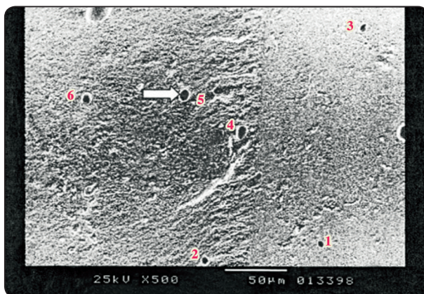
Fig. (6): SEM micrograph of the fractured surface of Grandio after 6 weeks water storage showing multiple filler dislodgement and presence of internal pores (Sites 1-6).
