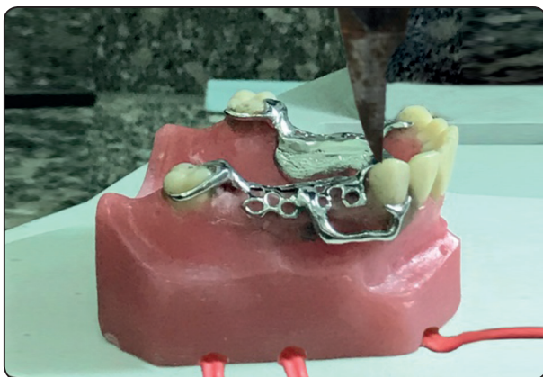
Fig. (2) Acrylic model with load applicator bar of the Universal Testing Machine
