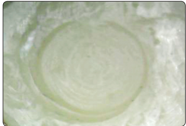
Fig. (2) Cohesive failure
