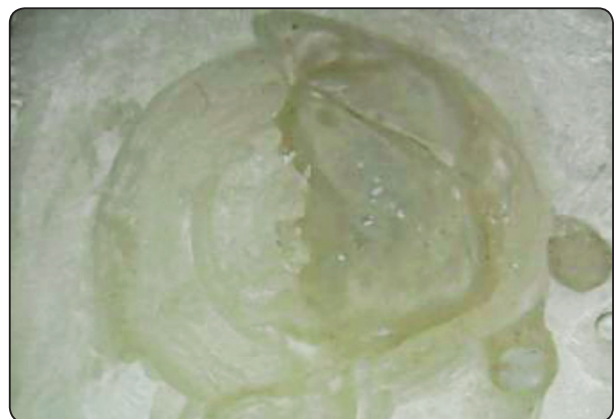
Fig. (3) Mixed failure
