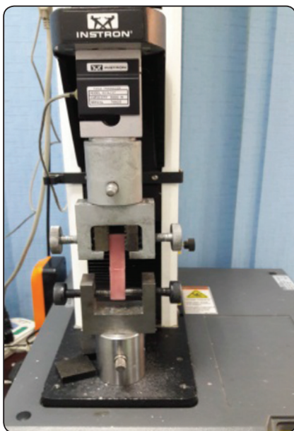
Acrylic samples fixed to universal testing machine
