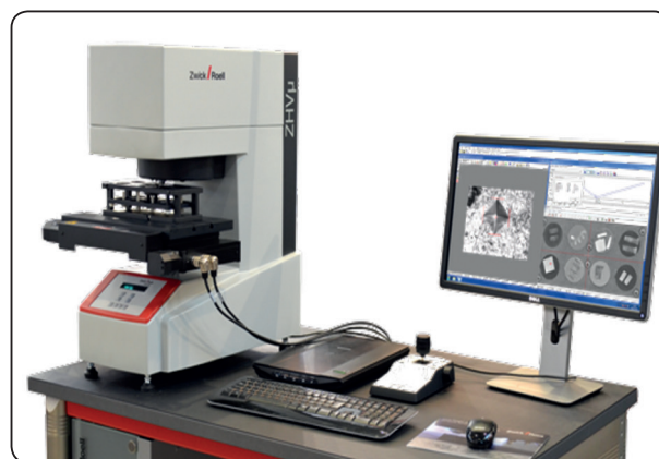
Fig. (2) Digital Microhardness Tester used for determination of hardness.
