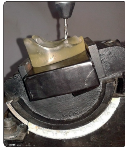
Fig. (1) The drill at the premolar region is 15° to a line drawn perpendicular to the occlusal plane.
