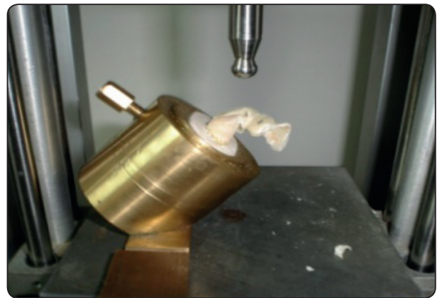
Fig. (4) Delaminated Fracture of the BioHPP specimen.
