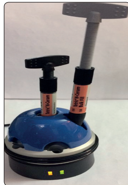
Fig. (1) Preheating of composite syringes in Calset device at (37-68°C)
