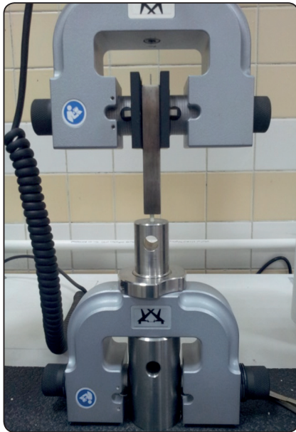
Fig. (2) The specimen in position in the Instron testing machine for compressive strength testing.
