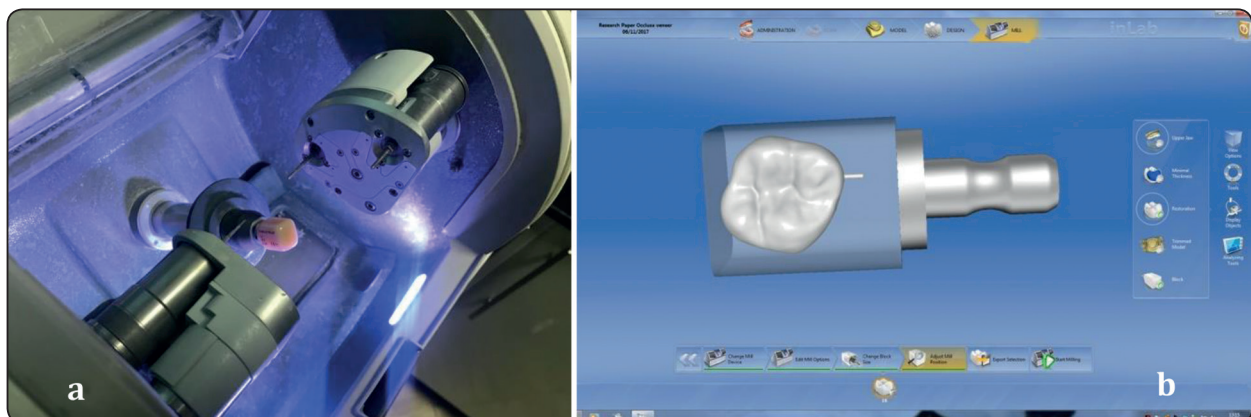
Fig. (9) The Celtra ceramic block secured in place in the milling machine (a). Virtual occlusal veneer design embedded in the block ready to start the milling process (b).
