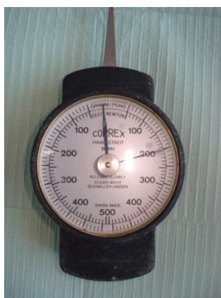
Figure 5: Correx tension gauge for retraction force measurement
