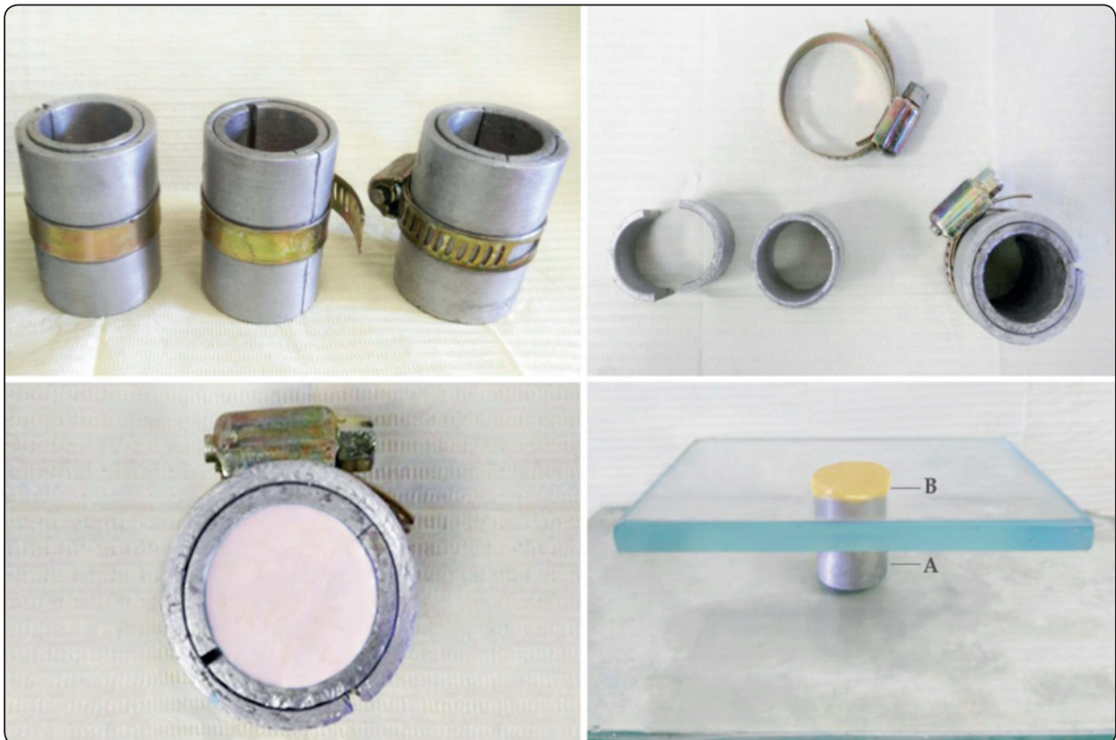
Fig (1): Cylindrical mold, lower ring (A) for tissue conditioner material and upper ring (B) to receive stone material.
