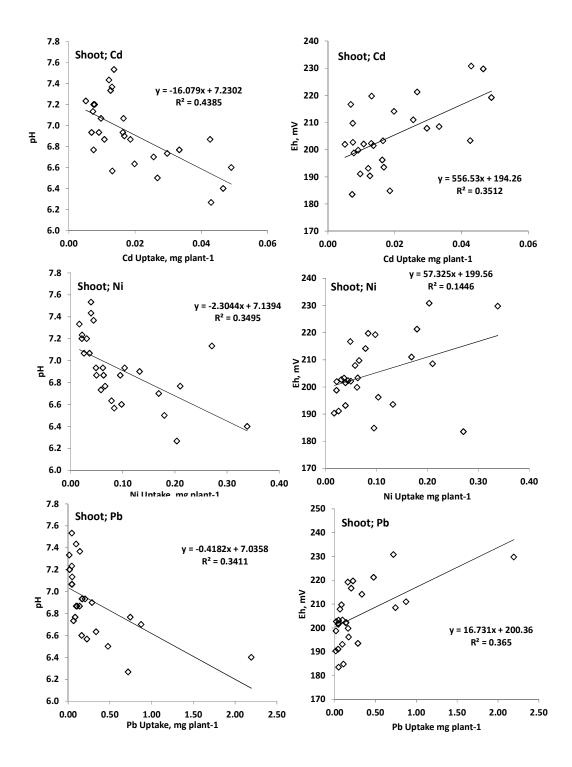
Fig. (3): Influence of pH and Eh (mV) of the soil-water system on Cd, Ni and Pb (mg plant<sup>-1</sup>) taken up by shoots of paper reed plant under using of heavy metal enriched water.
