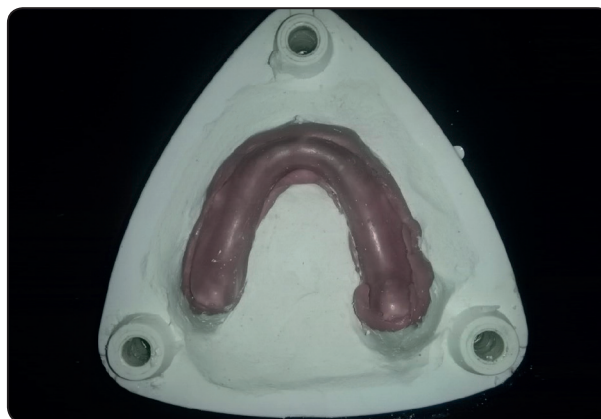
Fig. (2) Mold created in the die portion for the high impact microwave-cured mandibular acrylic resin denture bases.
