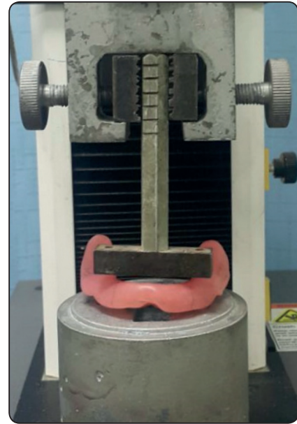
Fig. (3) Mandibular denture base mounted on a computer controlled testing machine subjected to compressive forces on its polished surface by a metallic loading bar at the canine-premolar regions bilaterally.
