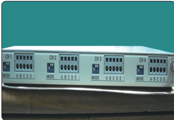
Fig (5) Multichannel Strain meter
