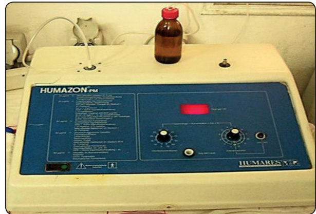
Fig. 4. Ozone generator ( Humazon ® Promedic, Humares GmbH, Bruchsal, Germany) and the fed glass bottle connected via inlet and outlet tubes.
