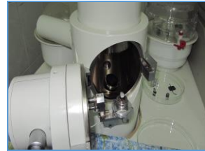
Fig 16: Specimen mounted on the electron microscope
