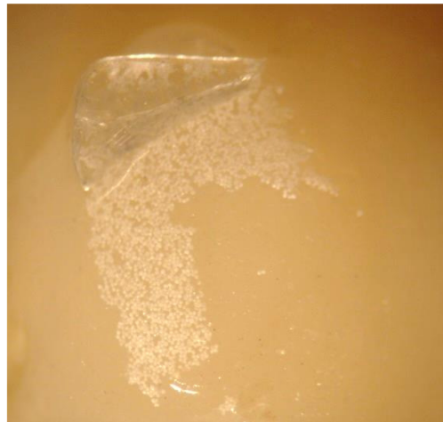
Figure 2: Stereomicroscope image showing enamel surface fragment of ceramic bracket.
