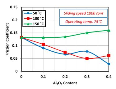
Fig. 10 Comparison of the effect of mixing temperature on the friction coefficient at different Al<sub>2</sub>O<sub>3</sub> content
