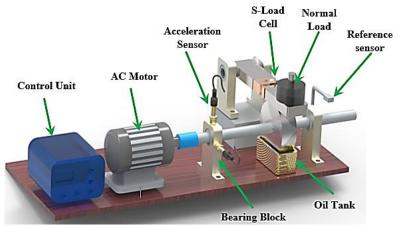
Fig. 1 Representation of the tribometer and vibration test rig.
