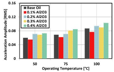
Fig. 16 Comparison between different operating temperatures for oil at 150°C mixed temperature.
