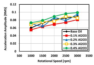
Fig. 15 Acceleration amplitude [RMS] with different rotational speed for Al<sub>2</sub>O<sub>3</sub> mixed at 150°C temperature and operated at 50°C temperature.
