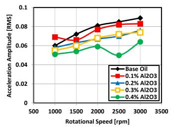
Fig. 11 Acceleration Amplitude [RMS] with different rotational speed for Al<sub>2</sub>O<sub>3</sub> mixed at 50°C temperature and operating at 50°C temperature.
