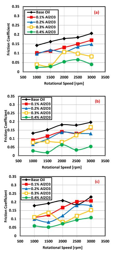
Fig. 4 Friction coefficient with different rotational speed for Al<sub>2</sub>O<sub>3</sub> mixed at temperature 50°C and operating at temperatures (a) 50°C, (b) 75°C and (c) 100°C.
