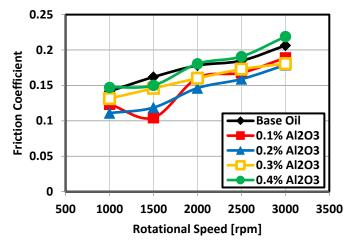
Fig. 8 Friction coefficient with different rotational speed for Al<sub>2</sub>O<sub>3</sub> mixed at 150°C temperature and operating at 50°C temperature.
