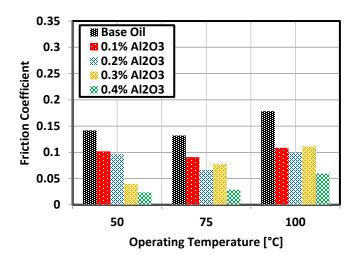
Fig. 5 Friction coefficient observed at different operating temperatures at 50°C mixed temperature.
