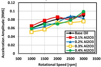
Fig. 13 Acceleration amplitude [RMS] with different rotational speed for Al<sub>2</sub>O<sub>3</sub> mixed at 100°C temperature and operating at 50°C temperature.
