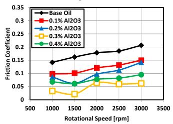
Fig. 6 Friction coefficient Friction coefficient with different Rotational Speed for Al<sub>2</sub>O<sub>3</sub> mixed at 100°C temperature and operating at 50°C temperature.
