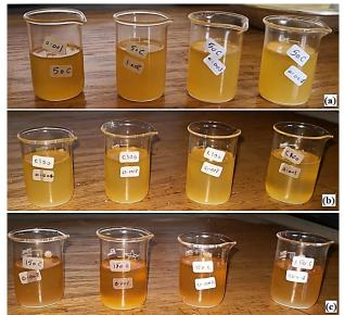
Fig. 2 Oil samples mixed with Al<sub>2</sub>O<sub>3</sub> nanoparticles at temperature (a) 50°C, (b) 100°C and (c) 150°C.
