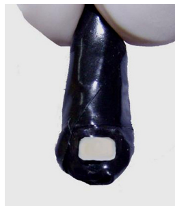
Fig 1: The tooth wrapped with an adhesive tape leaving a window the size of an orthodontic bracket base
