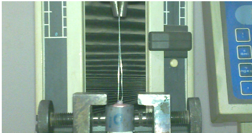
Figure 1: Specimen fixed to testing machine for assessment of fracture load of the self ligature assembly.
