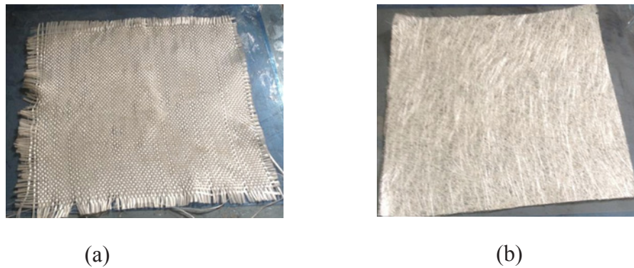
Fig. 1. Types of reinforcement (a) 2D plain woven glass (b) chopped strand glass mats.
