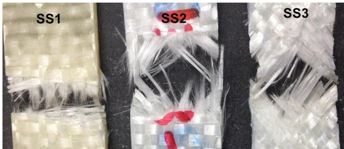
Fig. 3. Top view of failure of unnotched specimens with different stacking sequences.
