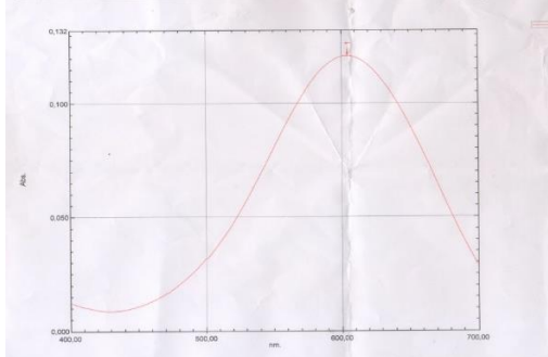
Fig.2 UV-visible spectrum of DCPIP versus the reagent blank.
