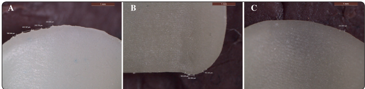
Fig. (7) A: e.max/2-step milling/ Cervical margin. B: Empress CAD/2-step milling/ incisal periphery. C: Vita Enamic/2-step milling/ cervical margin
