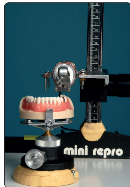
Fig. (1) Custom-made setup for measurements standardization using the Tooth Pressure Meter
