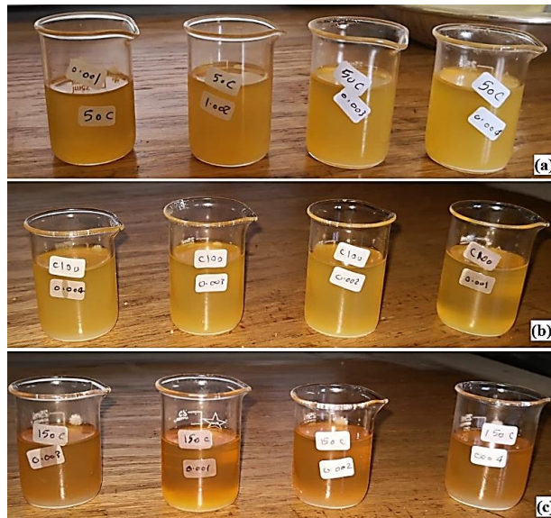
Fig. 2 Oil samples mixed with \text{Al}_2\text{O}_3 nanoparticles at temperature (a) 50°C, (b) 100°C and (c) 150°C.
