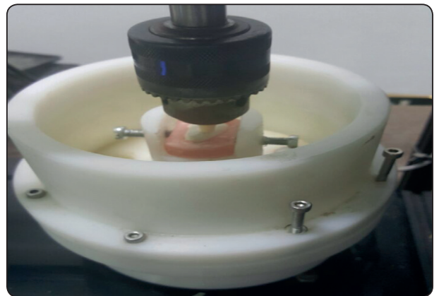
Fig. (2) showing shows the ROBOTA chewing simulator chamber with loaded sample.
