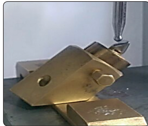
Fig. (1): Specimen loaded in the universal testing machine for testing fracture strength.
