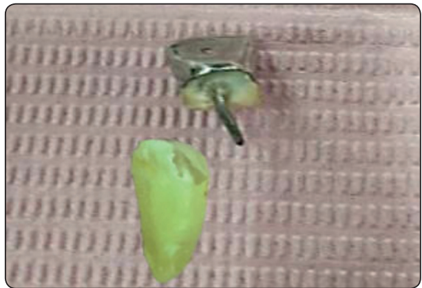
Fig. (4) Mid root fracture Metal post Gp.A1.
