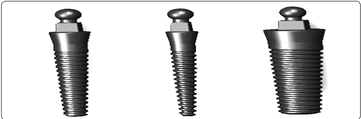
Fig. (1): Model of analyzed implants: Right: Standard \varnothing 3.8 mm implant, Left: \varnothing 2.4mm mini-implant, Middle: \varnothing 1.8 mm mini-implant
