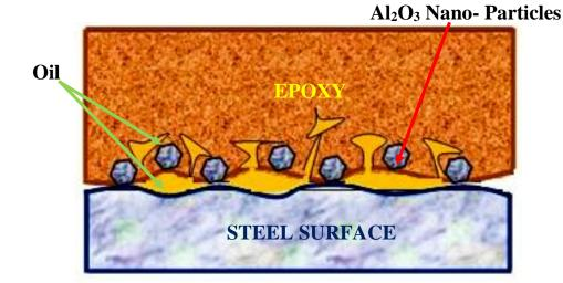
Fig. 5 The oil cover contact surface and reduce the adhesion between epoxy and steel surface
