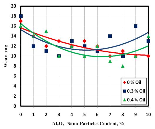
Fig. 11 Wear of epoxy test specimens filled by Al<sub>2</sub>O<sub>3</sub> and paraffin oil.
