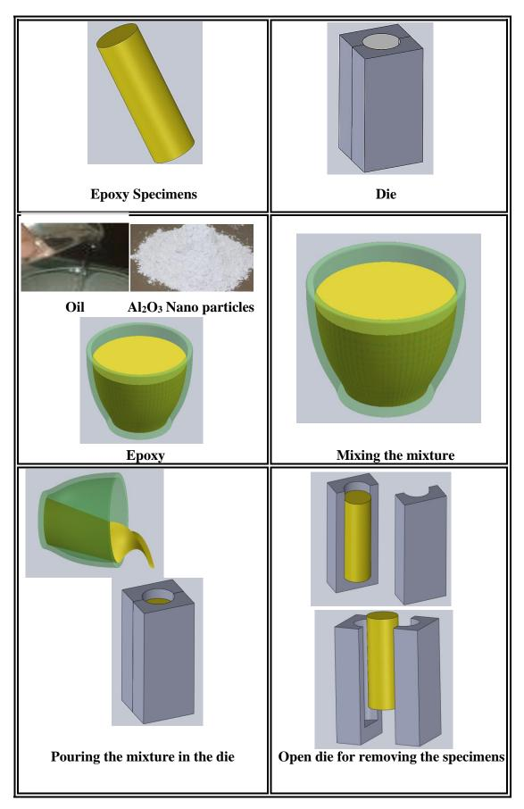
Fig. 2 Steps of test specimens preparation.
