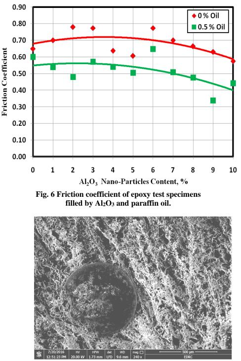
Fig. 7 The oil covers the contact area.
