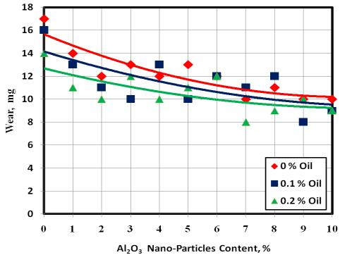
Fig. 9 Wear of epoxy test specimens filled by Al<sub>2</sub>O<sub>3</sub> and paraffin oil.
