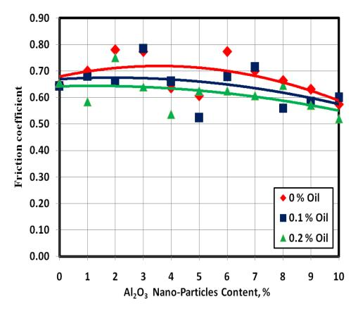
Fig. 3 Friction coefficient of epoxy test specimens filled by Al<sub>2</sub>O<sub>3</sub> and paraffin oil.
