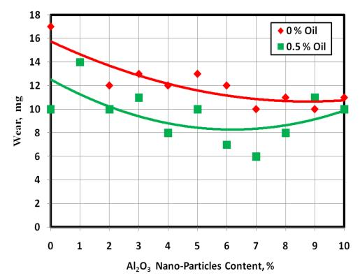
Fig. 12 Wear of epoxy test specimens filled by Al<sub>2</sub>O<sub>3</sub> and paraffin oil.
