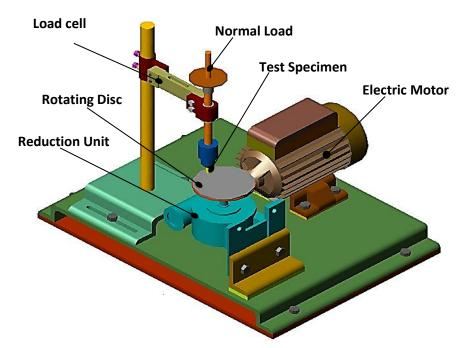
Fig. 1 Arrangement of friction test rig.
