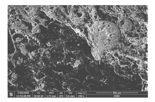
Fig. 8 The oil covers the contact area.
