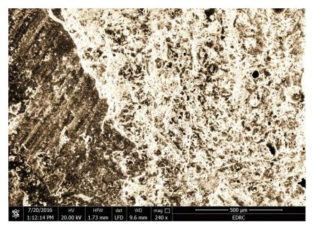
Fig. 10 Cavities from leakage the oil from test specimens
