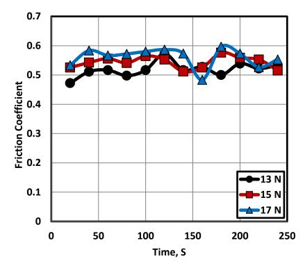
Fig. 15 Friction coefficient of epoxy composites filled by 22 wt. % copper, 56 wt. % rubber, 2 wt. % sand.
