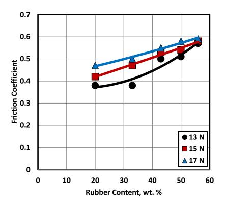
Fig. 17 Friction coefficient displayed by epoxy composites filled by rubber, copper and sand.
