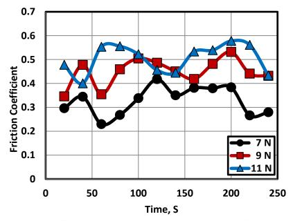
Fig. 2 Friction coefficient displayed by epoxy composites filled by rubber.
