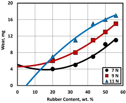
Fig. 18 Wear displayed by epoxy composites filled by rubber, copper and sand.
