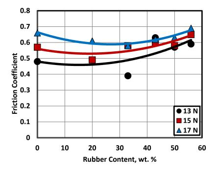
Fig. 5 Friction coefficient displayed by epoxy composites filled by rubber.
