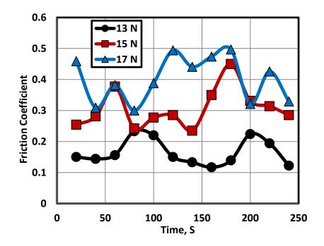
Fig. 9 Friction coefficient displayed by epoxy composites filled by rubber and copper.
