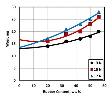
Fig. 13 Wear displayed by epoxy composites filled by rubber and copper.
