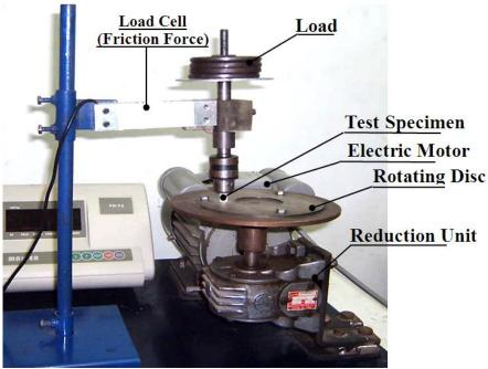
Fig. 1 Test rig used in measuring friction and wear.
