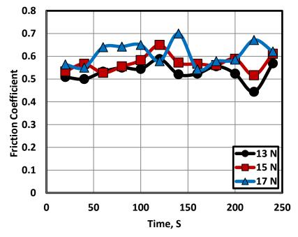
Fig. 3 Friction coefficient displayed by epoxy composites filled by 56 wt. % rubber.
