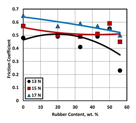
Fig. 11 Friction coefficient displayed by epoxy composites filled by rubber and copper.
