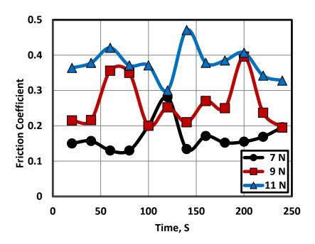
Fig. 8 Friction coefficient displayed by epoxy composites filled by rubber and copper.
