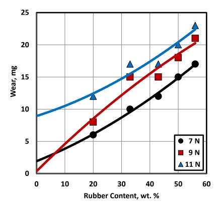
Fig. 12 Wear displayed by epoxy composites filled by rubber and copper.
