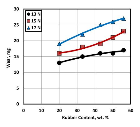
Fig. 7 Wear displayed by epoxy composites filled by rubber.
