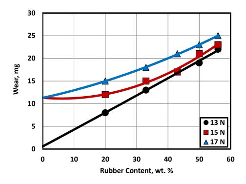
Fig. 19 Wear displayed by epoxy composites filled by rubber, copper and sand.
