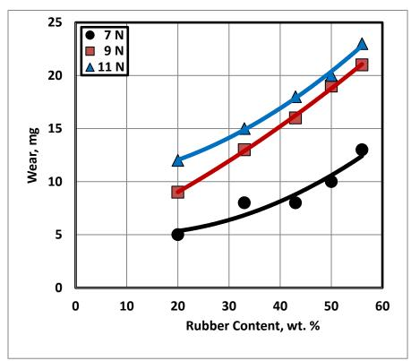
Fig. 6 Wear displayed by epoxy composites filled by rubber.
