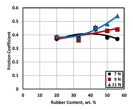
Fig. 16 Friction coefficient displayed by epoxy composites filled by rubber, copper and sand.
