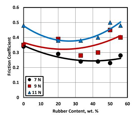
Fig. 10 Friction coefficient displayed by epoxy composites filled by rubber and copper.
