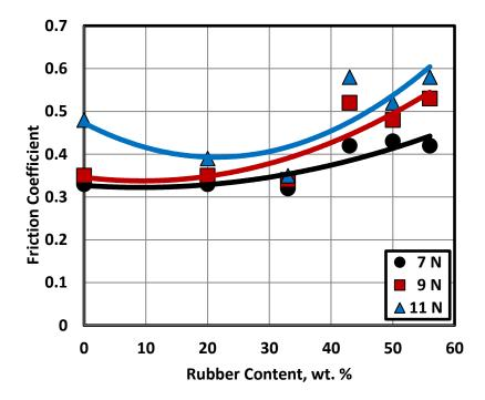
Fig. 4 Friction coefficient displayed by epoxy composites filled by rubber.
