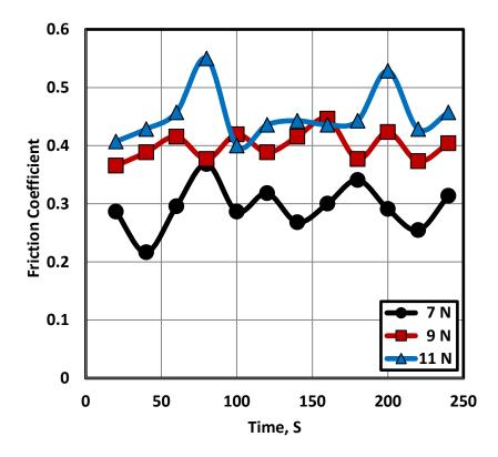
Fig. 14 Friction coefficient of epoxy composites filled by 22 wt. % copper, 56 wt. % rubber and 2.0 wt. sand.
