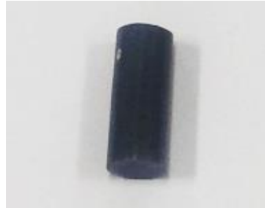
Fig.5 Sample of PMMA material reinforced with MWCNTs.
