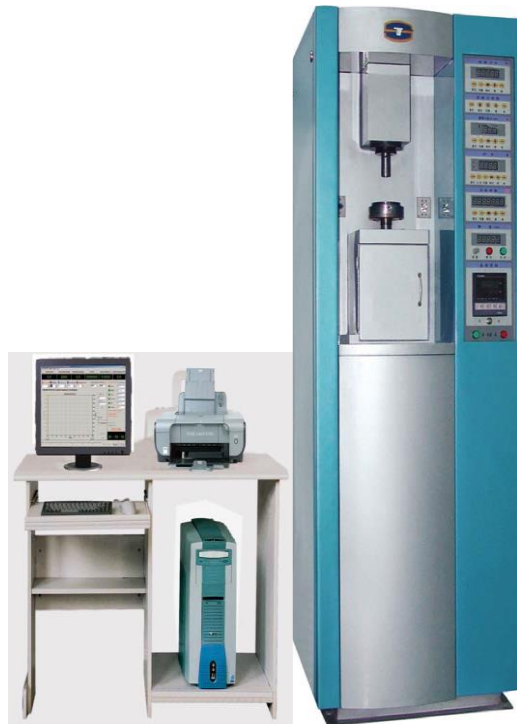
Fig. 1 Vertical universal friction and wear testing machine, (MM-W1A).
