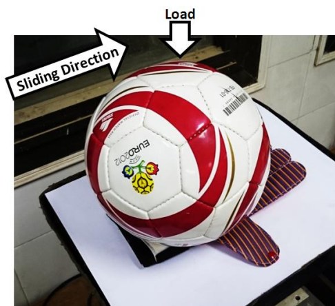
Fig. 2 Measurement of friction force between the football and the glove.
