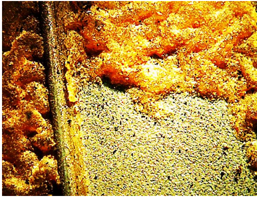
Fig. 6 Flow of polyurethane around the steel wire.
