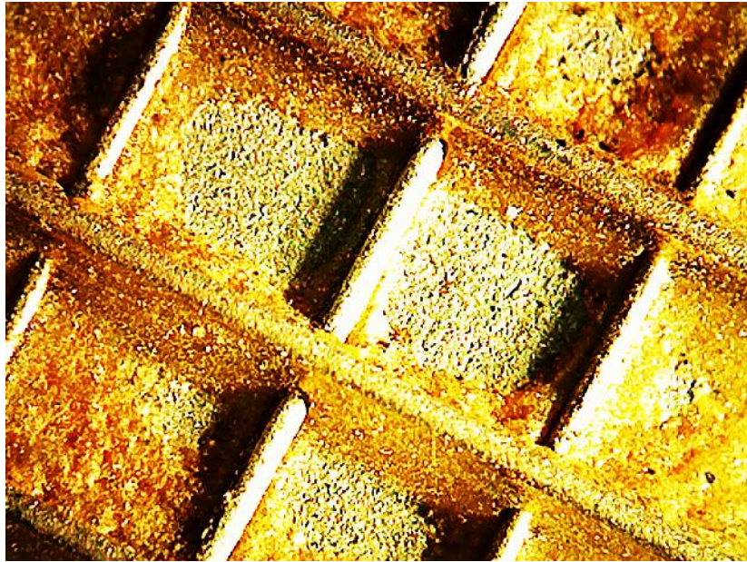
Fig. 10 Accumulation of polyurethane to the sides of steel wire.
