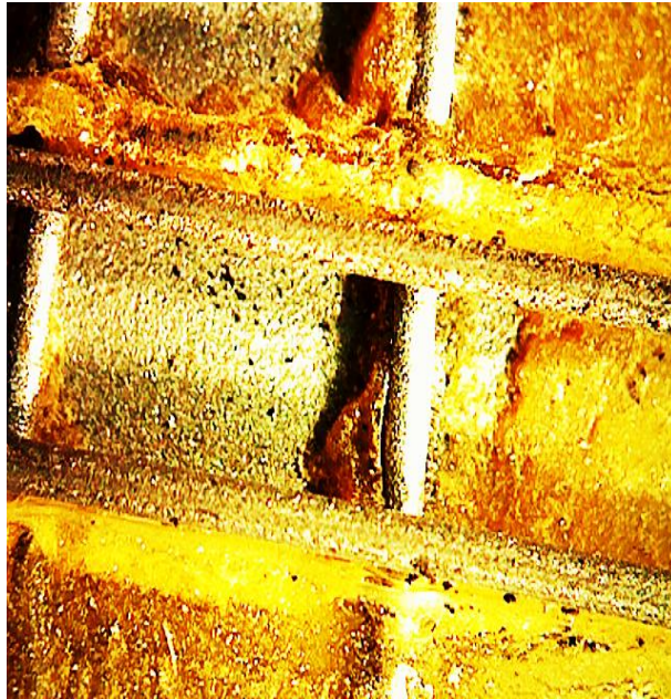
Fig. 12 Erosion of the test specimen reinforced by gridded wires.
