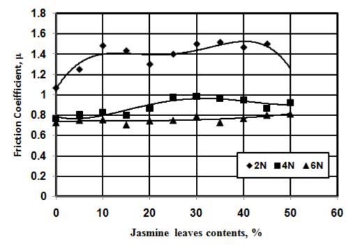
Fig. 7 Effect of soft jasmine leaves particles on the friction coefficient of polyester composites.
