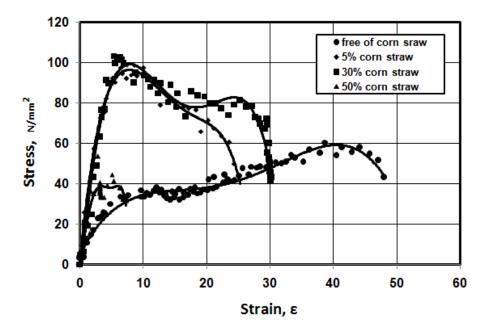
Fig. 5 Effect of coarse corn straw particles on the stress-strain curve of polyester composites.
