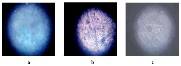
Fig. 1 a) Unfilled polyester, b) Polyester reinforced by soft particles and c) Polyester reinforced by coarse particles.
