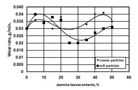
Fig. 9 Effect of jasmine leaves particles on the wear rate of polyester composites.
