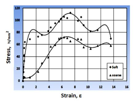
Fig. 11 Stress – strain curve for polyester composite filled with 5 wt. % jasmine leaves.
