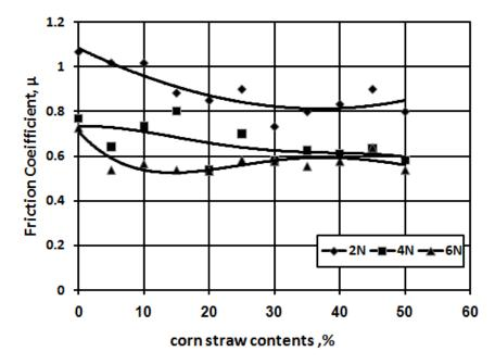
Fig. 2 Effect of coarse corn straw particles on the friction coefficient of polyester composites.
