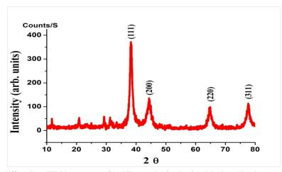
Fig. 7. The X-ray diffraction (XRD) patterns of AuNPs synthesized using Moricandia nitens aerial parts extract.
