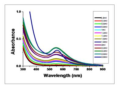
Fig. 1. Uv-vis spectra of gold nanoparticles using constant HAuCl4 concentration (1.4x10<sup>-4</sup>M) and different Moricandia nitens aerial parts extract concentrations.
