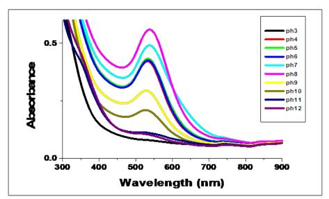
Fig. 4. Uv-Vis spectra of AuNP synthesized using 2.6 ml of Moricandia nitens aerial parts extract using HAuCl<sub>4</sub> at different pH of the extract (pH 3-12).
