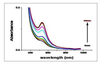
Fig. 3. UV–Vis spectra recorded from reduction of 1.4x10<sup>4</sup> M HAuCl<sub>4</sub> using 2.6 ml of Moricandia nitens aerial parts extract at various time intervals of 5 minutes for 40 minutes.
