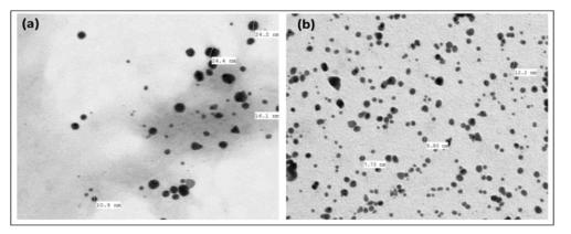
Fig. 2. TEM images of AuNPs synthesized using HAuCl4 (1.4x10<sup>-4</sup>M) and (a) 0.4ml and (b) 2.6 ml of Moricandia nitens aerial parts extract.
