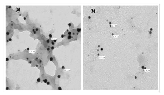
Fig. 5. TEM images of AuNPs (a) at pH4 and (b) at pH8 of plant extract.
