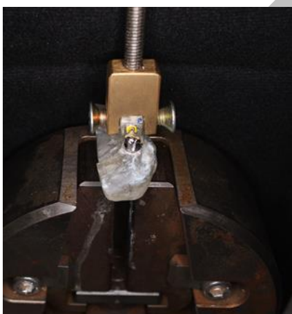
Figure (5): CAD/CAM bar (group 2) attached to universal testing machine.
