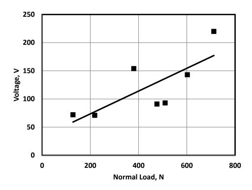
Fig. 8 Electric static charge of floor generated from its sliding against dry shoe sole.
