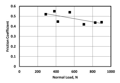
Fig. 9 Friction coefficient displayed by sliding of shoe against water wetted floor.
