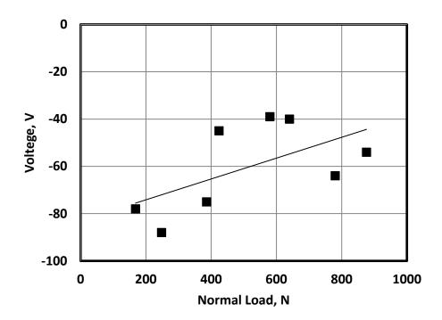
Fig. 12 Electric static charge of shoe generated from its sliding against water wetted floor.
