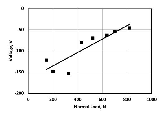
Fig. 5 Electric static charge of shoe generated from its contact and separation against dry floor.
