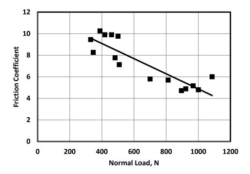
Fig. 4 Friction coefficient displayed by sliding of shoe against dry floor.
