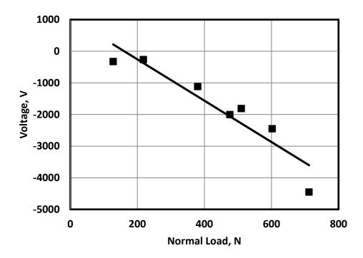
Fig. 7 Electric static charge of shoe generated from its sliding against dry floor.
