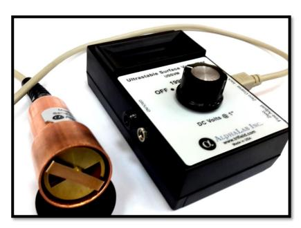
Fig. 1 Electrostatic field measuring device.
