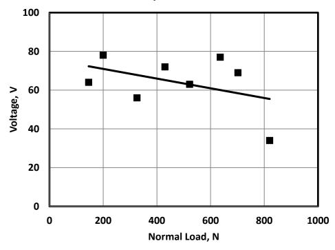
Fig. 6 Electric static charge of floor generated from its contact and separation against dry shoe sole.
