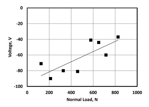
Fig. 10 Electric static charge of shoe generated from its contact and separation against water wetted floor.
