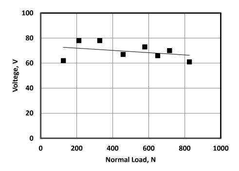
Fig. 11 Electric static charge of floor generated from its contact and separation against water wetted shoe sole.
