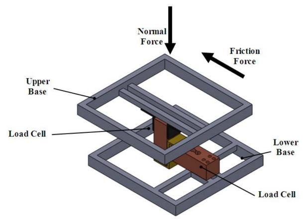
Fig. 2 Arrangement of the test rig.
