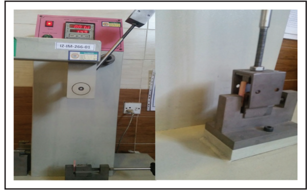
Fig. (3) Izod/Charpy Digital Impact tester during impact strength test
